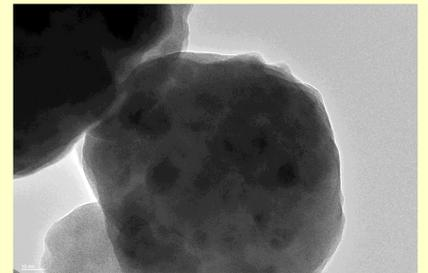
**As received sample:** spongy aspect with large numbers of pores and voids; average crystallite size about 10 nm. After hating 1h at the temperatures 600C and 900C crystallite growth was noticed up to 50 nm.
