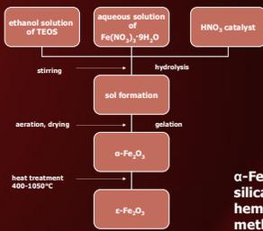
$\alpha$ - $Fe_2O_3$  nanoparticles (4nm) in a silica matrix containing 30 wt.% of hematite synthesized by the sol-gel method
