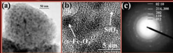
Transmission electron micrograph of  $\alpha$ - $Fe_2O_3/SiO_2$ : (a) silica grain with embedded  $\alpha$ - $Fe_2O_3$  nanoparticles; (b) high resolution image of selected grain region; (c) the SAED pattern of the same region
