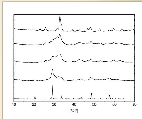
XRD patterns of the mixture of  $Y_2O_3$  and  $TiO_2$  powders and sponge  $Ti$ , in stoichiometric ratio for  $YTiO_3$ , milling for 0, 10, 30, 60 and 180 min.
